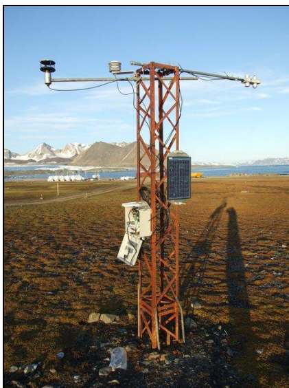
Photo 8.1. Radiation measuring station at Hornsund in 2008-2009 and net radiometer CNR1 Kipp&Zonen (Photo T. Budzik).
